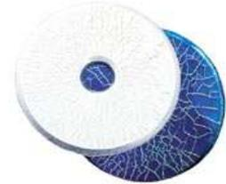
**Inspection** : The part is subjected to an intense magnetic flux, which is deviated by the presence of a defect. This escape attracts the particles of the product and the defects now are clearly visible as fluorescent or black lines.
